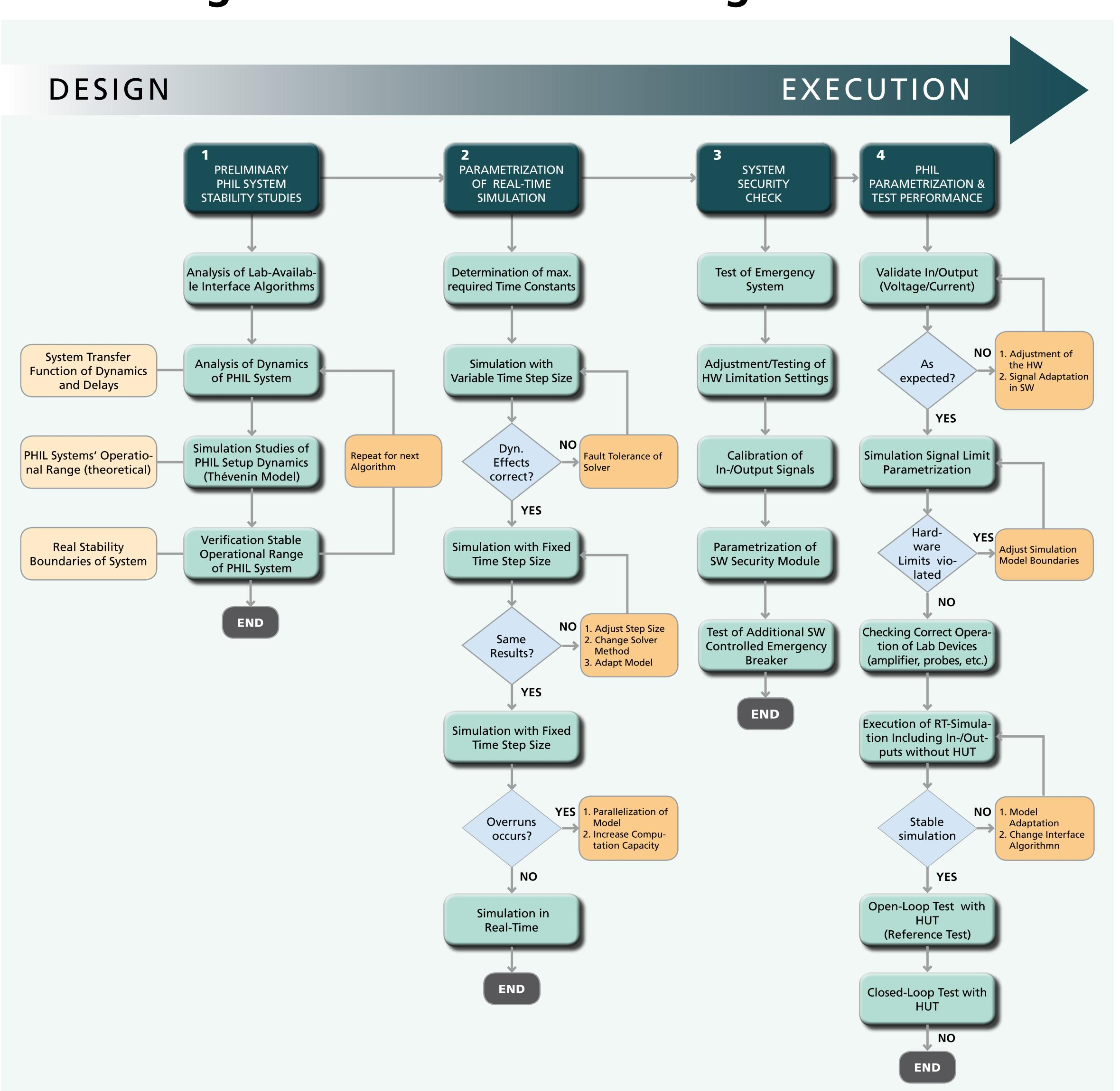
Process for the set-up and execution of PHIL experiments
